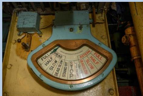
The engine room would confirm the new order by moving their lever to the matching position. The boiler room only had a telegraph repeater (shown above) and were not required to confirm an order. The fires in the boiler would be adjusted for the new speed and in the engine room the throttle valve would be adjusted to put more or less steam to the engine.
