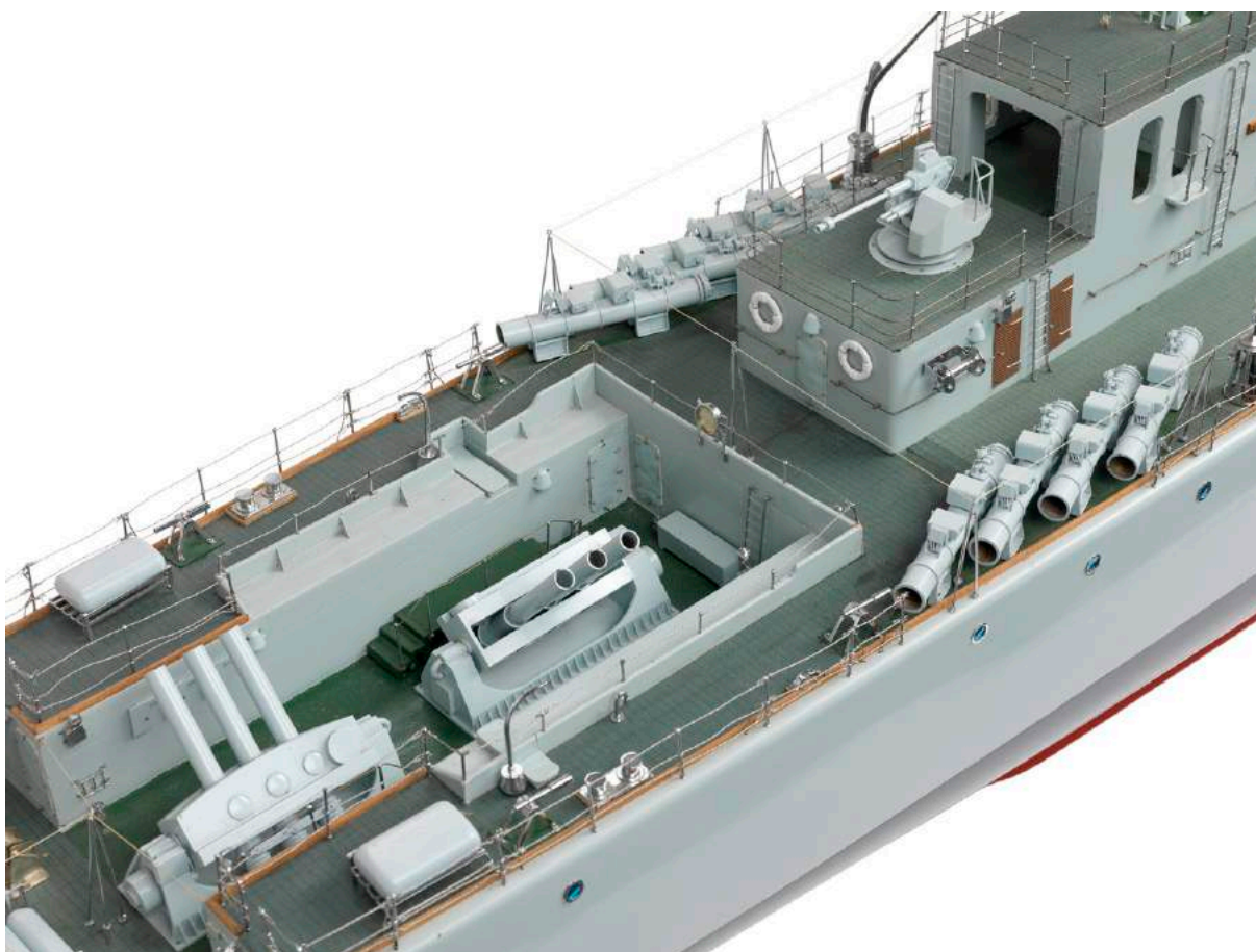
Ahead throwing weapons, a pair of three-barrel Limbo mortars on the frigate Londonderry of 1960. They could throw a pattern of six depth charges ahead of the ship.
