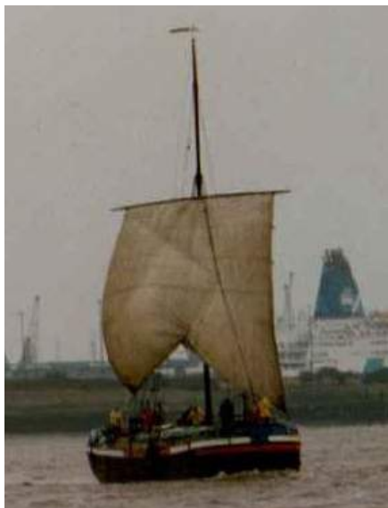
Single-masted square rig is extremely rare on modern vessels, but is seen here on the Comrade, a Humber keel of 1923.
