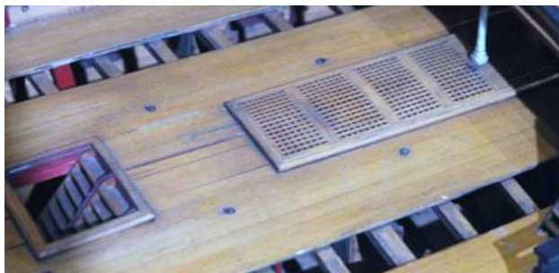
An open hatch used for a ladderway, with several hatches covered by gratings behind, on a mid-18th-century warship.
