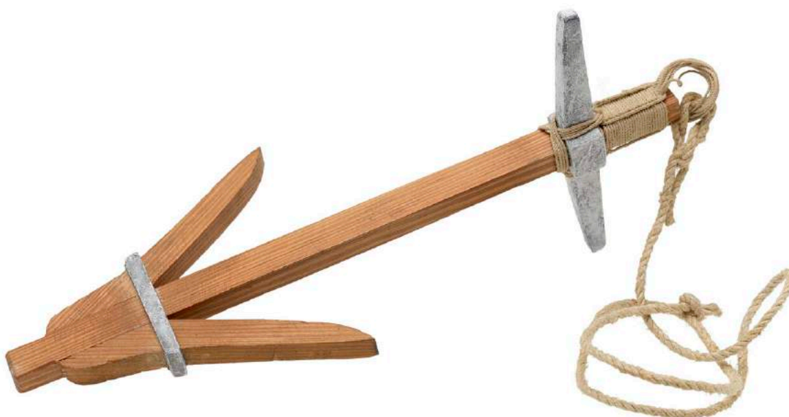
A modern model of a replica of an early 'killick' or small wooden anchor, with lead parts to make it sink.
