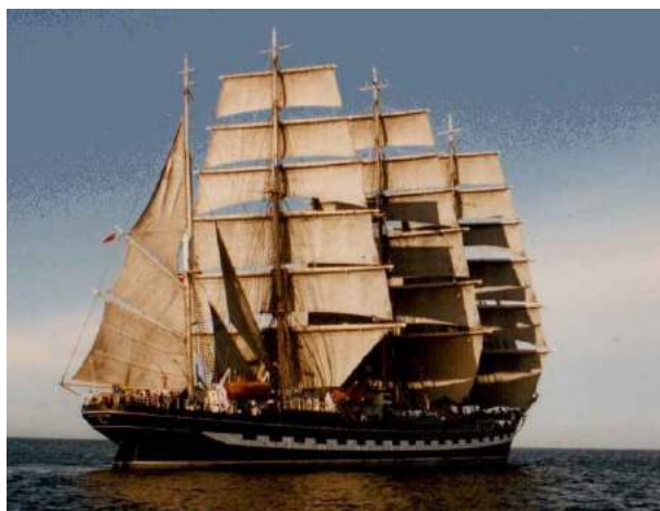
The Russian (ex-German) Kruzenshtern is a barque, square rigged on all masts except the after one.
