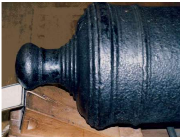
The rounded part or cascable of an Armstrong pattern gun © Brian Lavery
