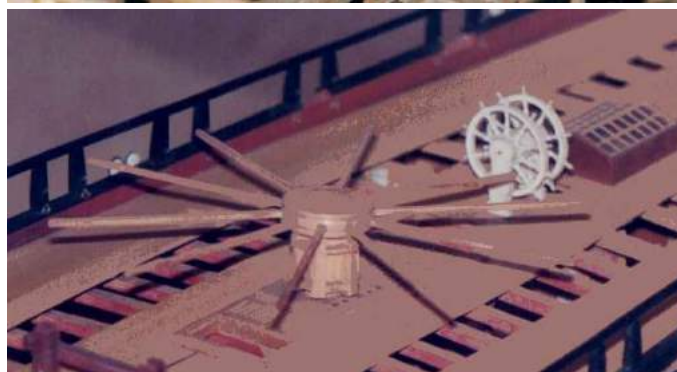
With the 'drumhead' capstan, each bar was set in a socket so they could all be kept at the same height. © Brian Lavery
