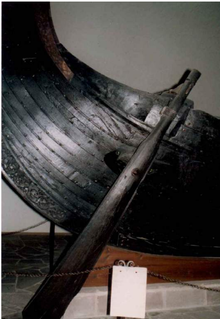
The side rudder of the Oseberg ship at the Viking Ship Museum in Oslo. © Brian Lavery
