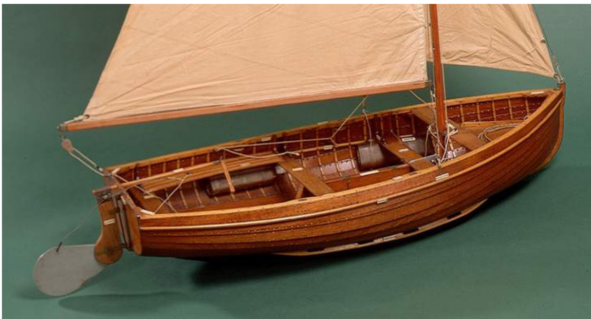
An RNSA (Royal Naval Sailing Association) dinghy from 1920 showing the tiller, rudder and rudder extension.
