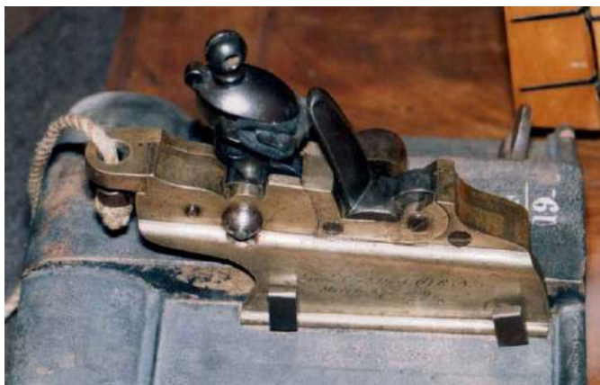
Locks similar to those used on muskets were often fitted to naval guns from about 1780.
