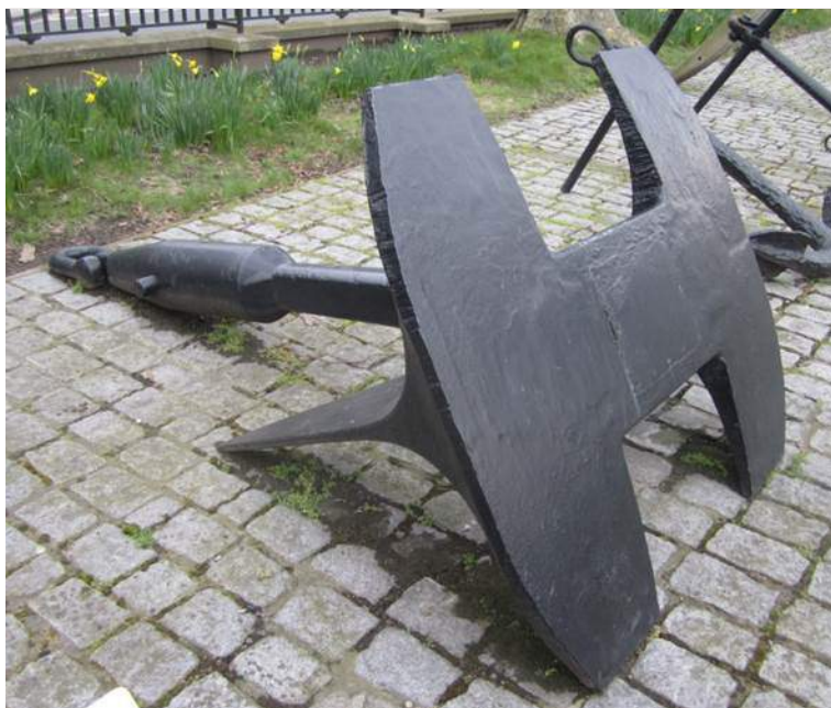
The anchor of the nuclear submarine Dreadnought of 1960 was designed to fit onto the shape of the hull.
