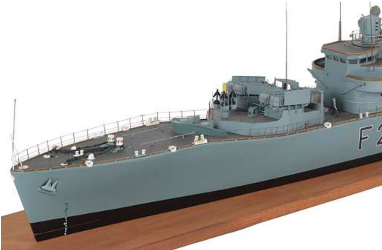
A model of the frigate Cleopatra in 1977, fitted with launchers for four Exocet anti-ship missiles and a quadruple launcher for Seacat short-range anti-aircraft missiles.
