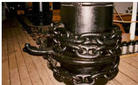
A bitt used for the chain cable of HMS Warrior of 1860.
