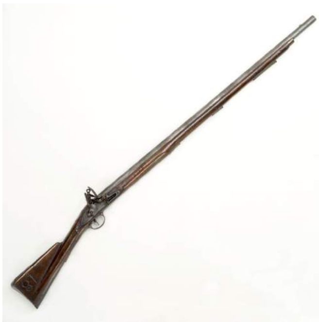
A standard 18th-century 'Brown Bess' flintlock musket. The naval version was similar to the army one, but more robust.
