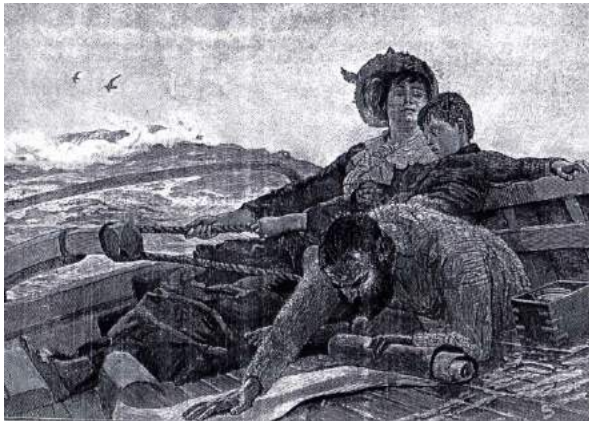
The marine artist W L Wyllie crosses the North Sea with family on his yacht Ladybird in 1888, showing the use of rope to get extra purchase on the tiller.
