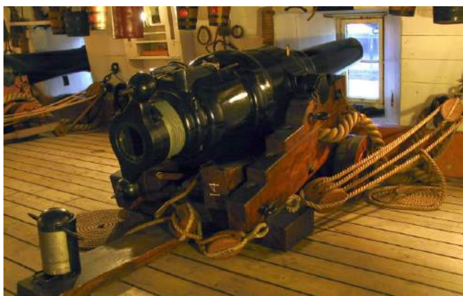
A 110-pounder gun, HMS Warrior of 1860. It was made in several parts and was breech-loading. However, it was too far ahead of its time and did not work well.
