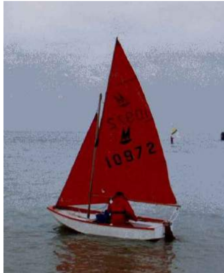
The 'sloop' rig with a mainsail and a single sail forward of the mast, seen here on the highly popular Mirror dinghy .
