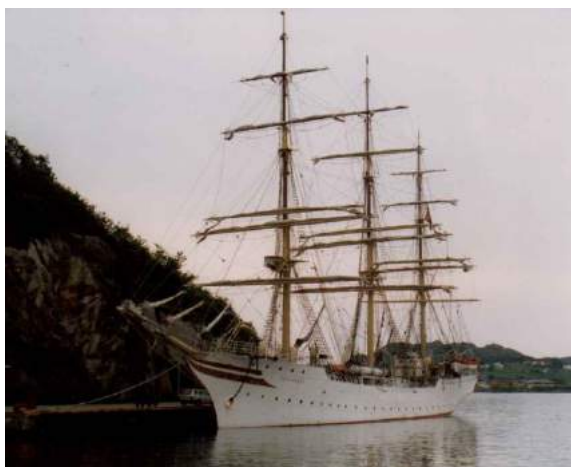
The Norwegian Sorlandet is a full-rigged ship, with three masts, all square rigged.
