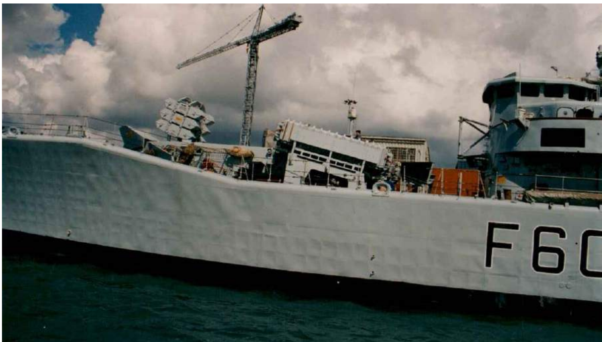
Exocet launchers just forward of the bridge on the frigate Jupiter in 1984, with six launchers for the Seawolf anti-aircraft missile just ahead.
