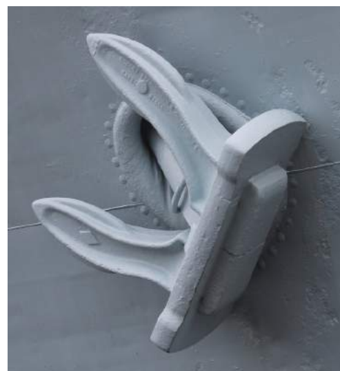
The stockless anchor of HMS Cavalier, a common type in the 20th century © Brian Lavery, with kind permission of Chatham Historic Dockyard Trust
