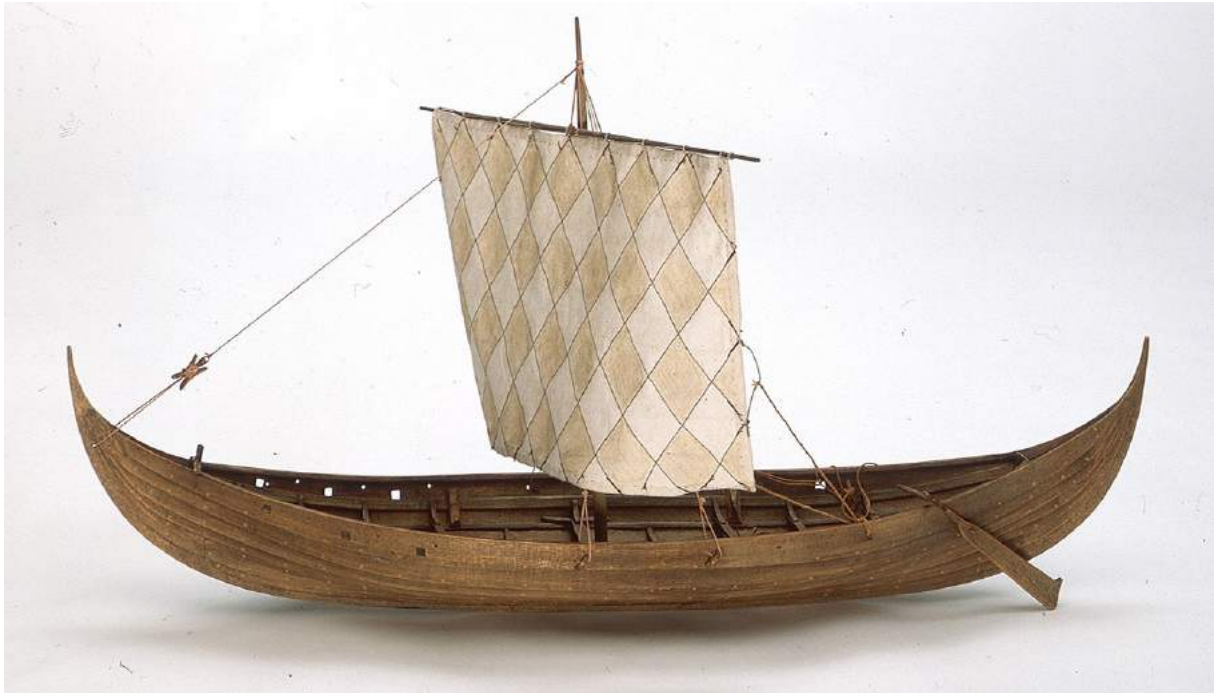
A model of the Viking ship known as Skuldelev 3, showing the side rudder. AOA0275 © National Maritime Museum, Greenwich, London
