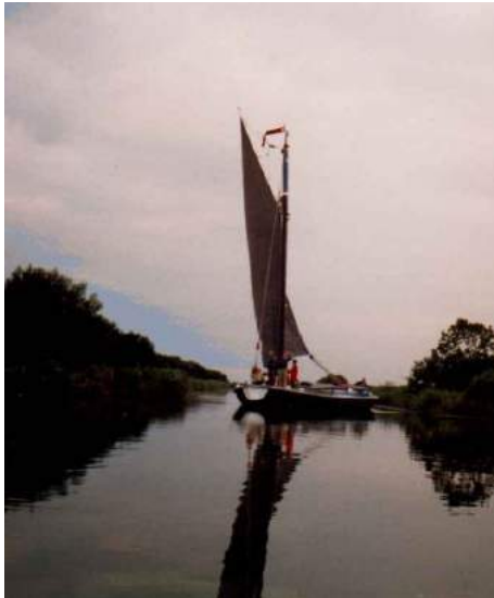
A Norfolk keel uses a single mast and sail.
