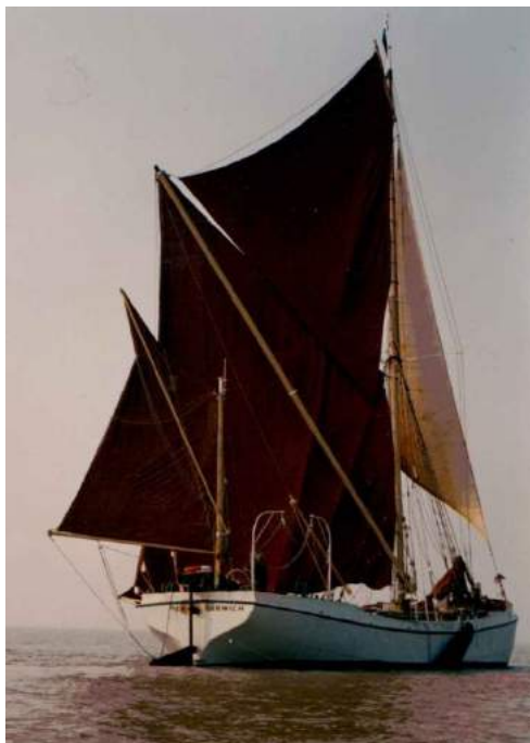
The yawl rig has a small mizzen mast well aft. The most common type in British waters is the Thames barge.
