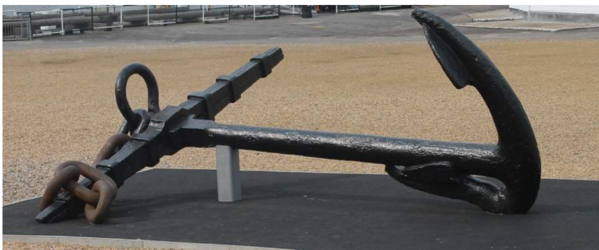
Another way of making a mooring anchor was to bend down one of the arms so that it was not a danger to shipping passing over it, as shown in this example in Chatham Historic Dockyard. Of course it would be the other way up when in use.
