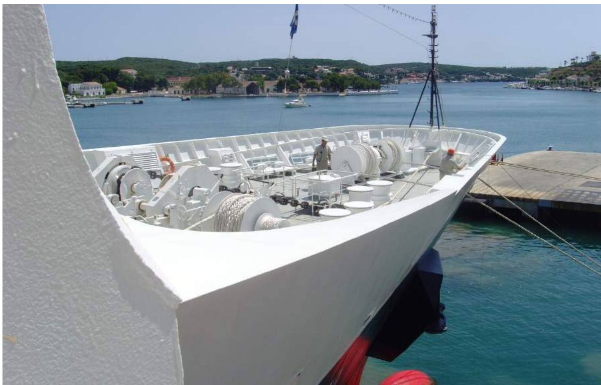
Coming alongside at Port Mahon in the cruise ship Minerva, showing the winches on the forecastle.
