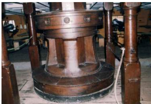
The lower part of the double capstan on HMS Victory © Brian Lavery
