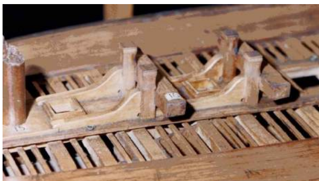
The bitts on the lower deck of an 18th-century ship, used to secure the anchor cable in the severest weather.
