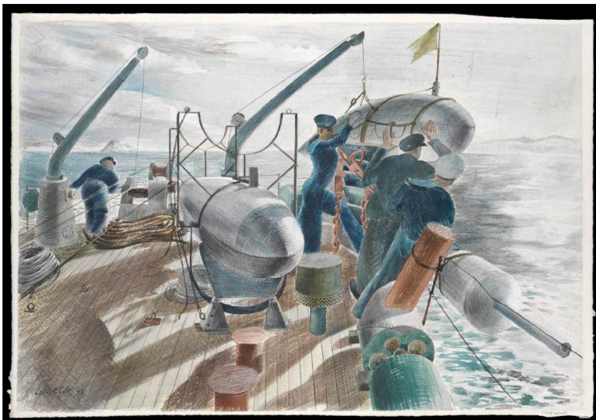
Minesweeping has been a major commitment of the Royal Navy since the First World War. In this 1943 picture by Leslie Cole the seamen are handling an Oropesa sweep, which keeps up the outer end of the wire used for sweeping.
