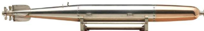
A model of the straighter type of torpedo used c 1910 - the Royal Gun Factory Mark V torpedo SLR2961 © National Maritime Museum, Greenwich, London, Phipps Hornby Collection
