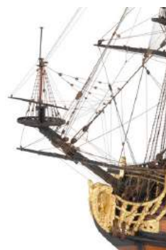
The spritsail topmast at the end of the bowsprit on a Navy Board model of c 1675.
