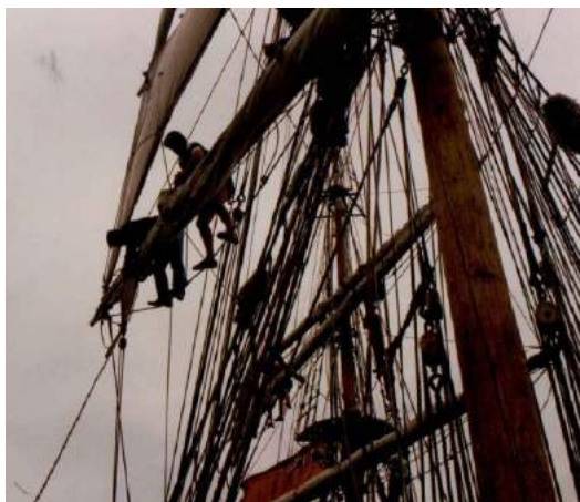
With square rigging it is usually necessary for crew to go aloft to loose and furl the sails.
