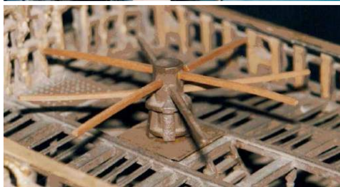
17th-century capstans had bars running all the way through, so they had to be set at different heights. © Brian Lavery, with kind permission of National Maritime Museum, Greenwich, London, (SLR0217)
