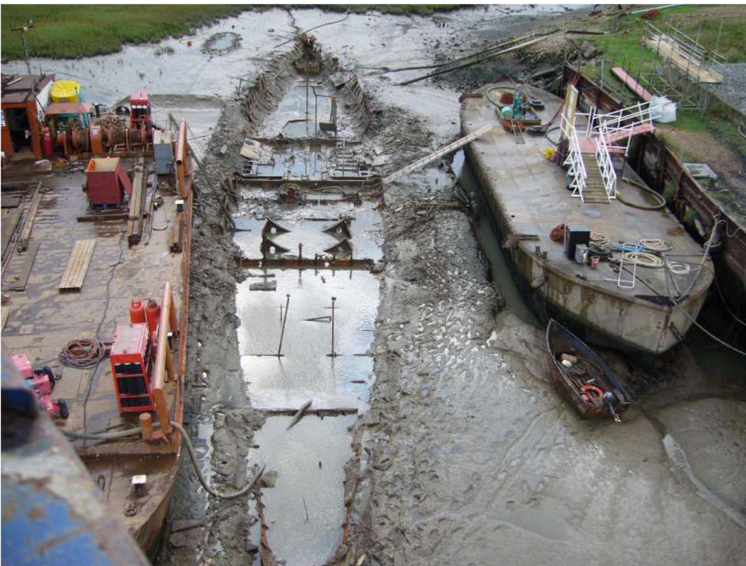
The final steps. Note boiler seats remaining in situ on bottom plating. New ones will be made to suit replacement boiler (W. Davies)
