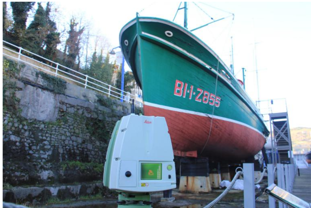
One of the stations for hull recording: the image created can be seen on the screen (J.M. Matés Luque)
