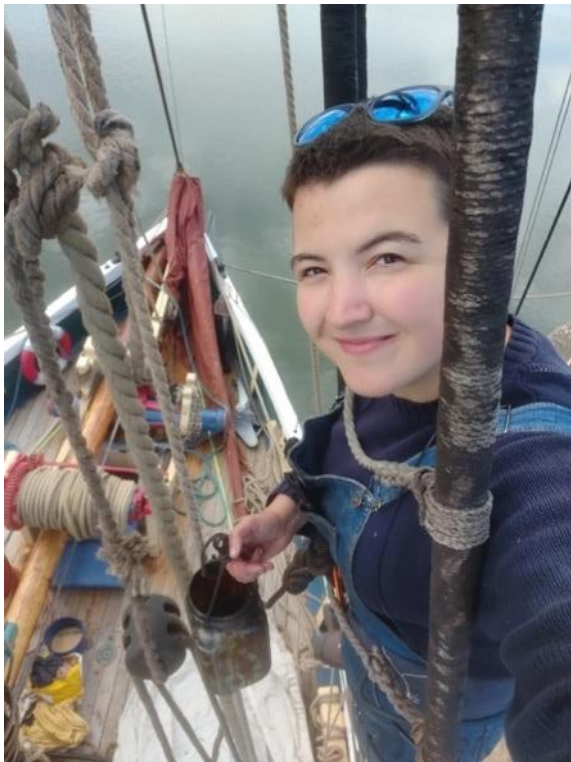
Oiling the shrouds with a Stockholm tar/linseed oil mix.
