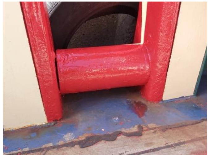
Unfortunately this roller has seized – it's part of the original fishing gear.
