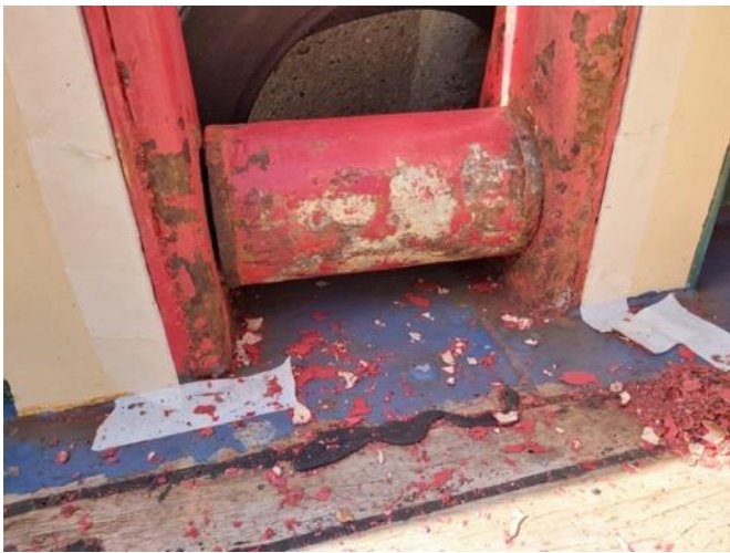
Unfortunately this roller has seized – it's part of the original fishing gear.
