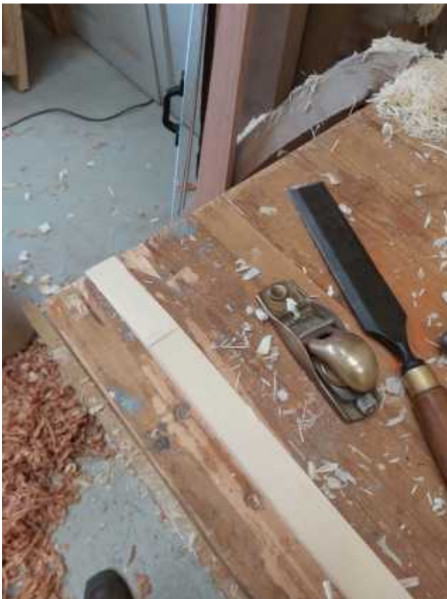
In order to make batons long enough for one of their projects, I cut some feather scarfs to join two shorter pieces together.
