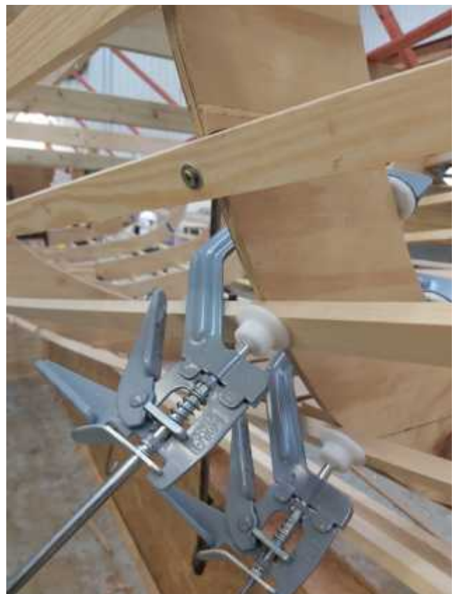
Attaching the new batons – this allows us to check for fair lines before the planks go on.
