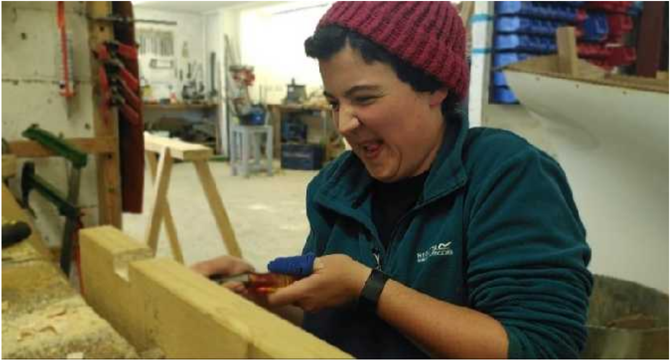
Ever the consummate professional – chiselling out some space for one of the legs in a sawhorse.
