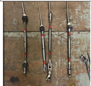
Old mismatched bottle screws from the shrouds
