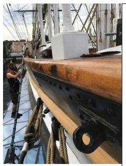
One thing that can be worked on with the public being back is the outer pin rail. In the images here we worked along the entire rail, from where it begins at the bow down and around the back of the poop deck. Often using harnesses to dangle over the edge as shown on the left, but where this was more difficult, we used steps to get up to the rail.
