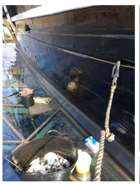
Once we had applied two coats of black paint to the hull, we then went about filling and fixing small cracks and breaks in the seams with caulk. At first, we applied caulk directly before smearing and cleaning with gloves and grimes. However, as I found this often resulted in a wide spread of caulk and in bad cases the removal of paint.
