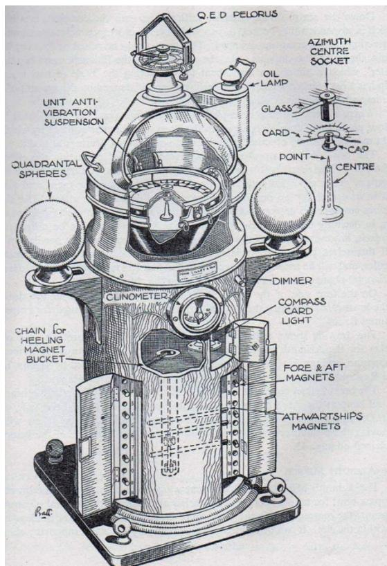
*Iron and steel ships usually had a pillar-like structure, with Newton's balls on either side. This example dates from 1939. The pelorus on top was used for taking bearings of objects.*
