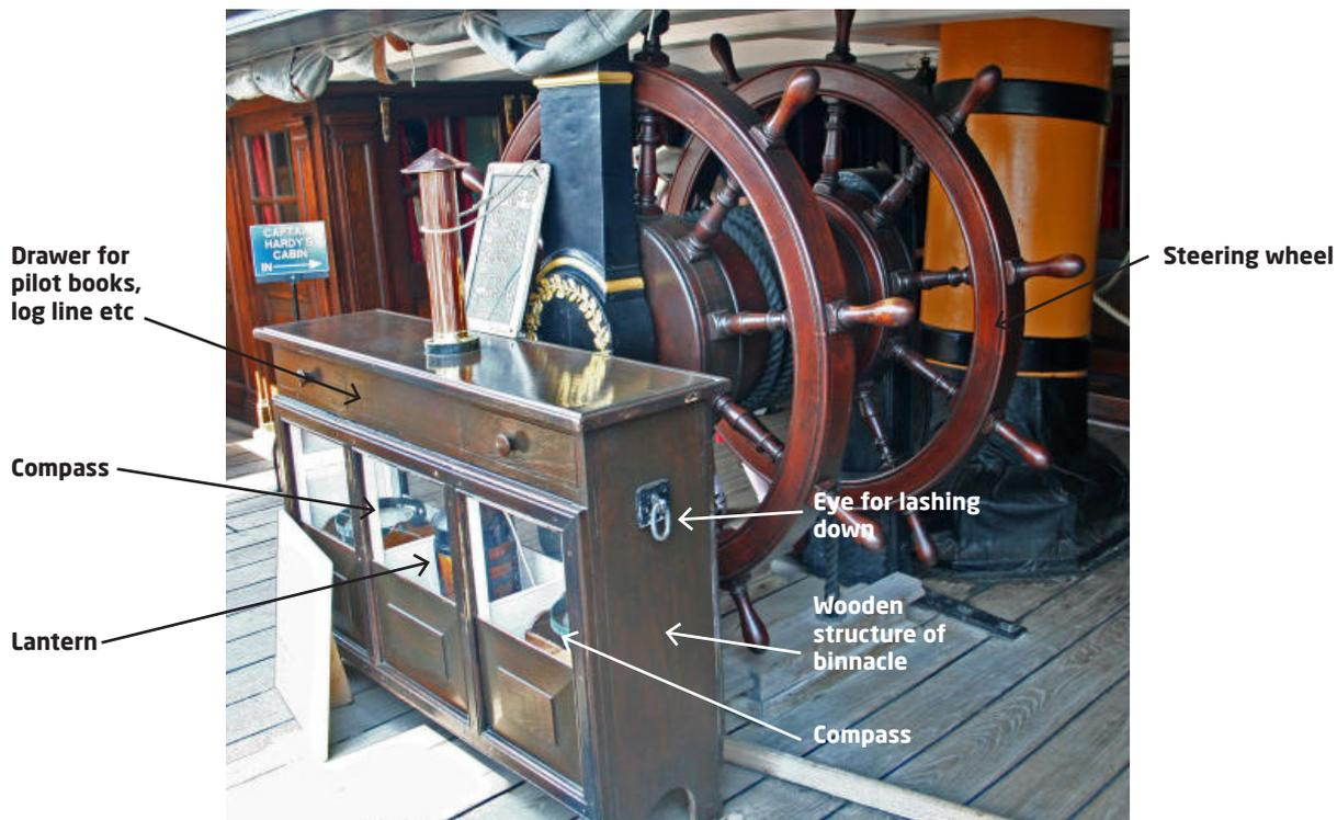
On deck, compasses were sited inside a structure known as the binnacle. In the age of sail this was a wooden box, shown here on *HMS Victory*. Since the helmsman might stand on either side of the wheel, there was a compass on each side, with a lantern between them for night-time use.
