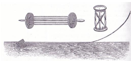
*A log and its line, the reel to which it is attached, and the sandglass used for timing.*
