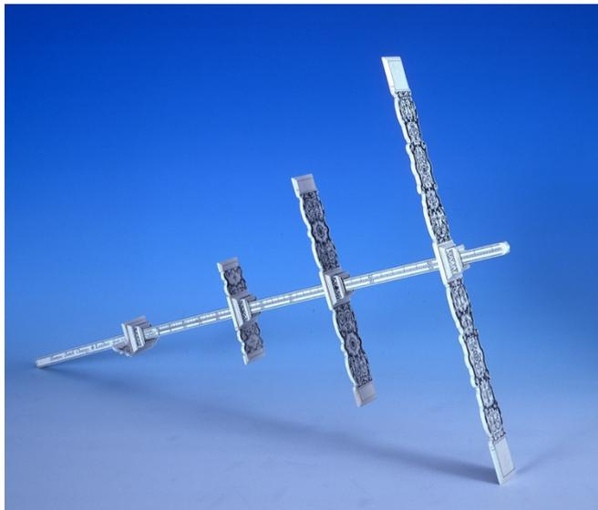
One of the most important issues in celestial navigation was to measure angles as accurately as possible. The cross staff used moveable vanes along a central staff – though only one was normally fitted at a given moment, according to the size of the angle. It could not be used to measure the angle of the sun without the danger of blindness. This example by Thomas Tuttell dates from around 1700.
