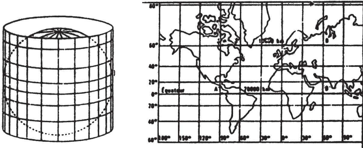
Most charts use Mercator's projection, showing a globe opened out and the distances expanded north and south away from the equator, from Chamber's Encyclopedia.
