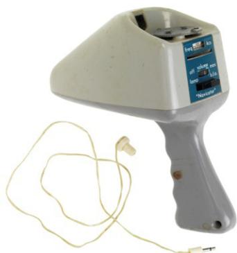
*The simplest aid was the radio direction finder which had to be pointed at a number of radio stations to take a fix. This example dates from around 1965.*
