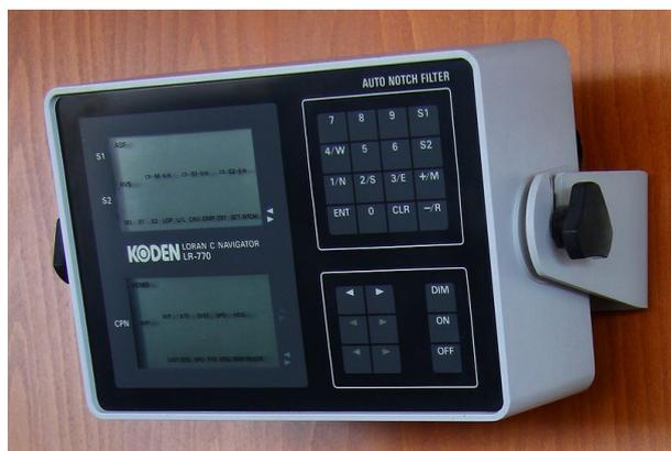
*Loran (LONg RANge Navigation) was an American system developed late in the Second World War. It was based on the time difference between the receipt of signals from a pair of radio transmitters. It has been run down since 2009 with most of its signals being shut off. Image:*
