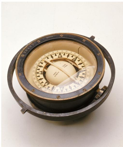
*The compass was usually placed inside a brass bowl and mounted on gimbals so that it stayed reasonably level in rough weather. This example dates from after 1920.*
