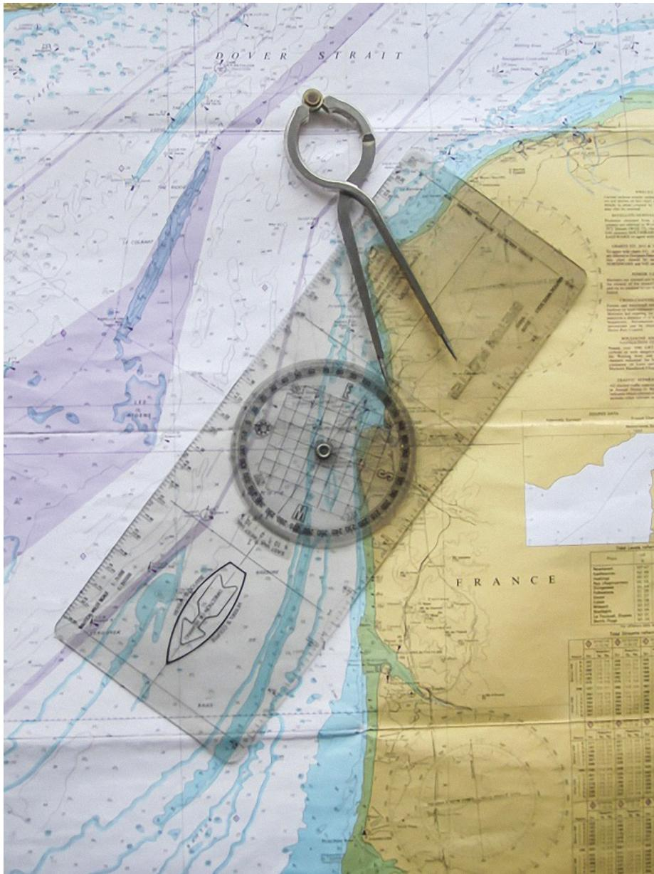
*The dividers were the standard means of measuring distances. The curved shape of the arms allows the instrument to be opened and closed with one hand. The Breton plotter is one of many instruments used to measure angles on the chart.*
