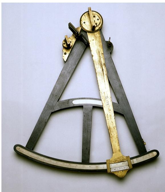
*The octant, often confusingly known as the quadrant, solved the problem more efficiently by using shades when looking at the sun. Though it only had an angle of 45 degrees or an eighth of a circle, this was doubled by the use of mirrors so that it could measure the angle of any celestial body. It was usually made of wood and ebony in this example by Troughton of around 1770, with features in brass.*
