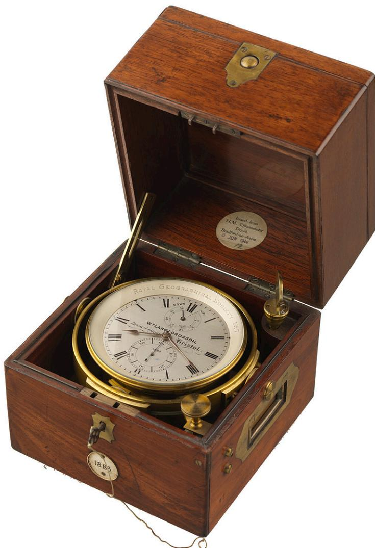
*Seamen need to measure the time for routine purposes such as timing the log and changing watches, but only a limited accuracy is needed for these purposes. For celestial navigation, especially for measuring longitude, it is essential to know the time far more accurately and any error over a period is likely to be cumulative. In the 18th century Thomas Harrison famously developed the chronometer as a very accurate clock for this purpose.*
