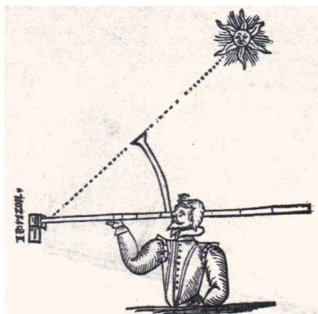
The backstaff solved the problem in a different way by having the observer's back to the sun. Its use is shown in this drawing of 1595.
