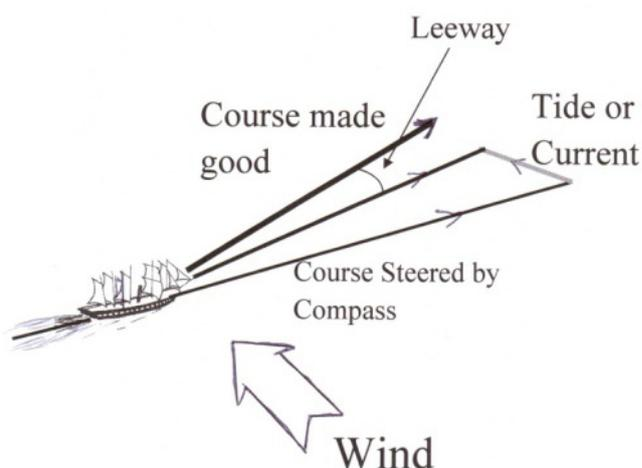
Moreover, in a sailing ship it is not always possible to steer a steady course over a period. This is calculated using a traverse board, in which the helmsman inserts a peg on a compass rose to record what he was able to steer during a short period, usually half an hour, which allows an estimate of the actual course to be calculated.
