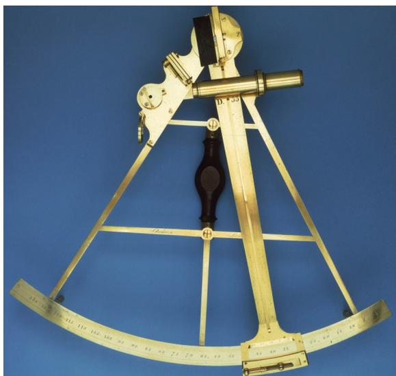
*The sextant was a development of the octant and the ultimate solution to the problems of measuring angles. It comprised a sixth of a circle or 60 degrees, increased to 120 degrees by mirrors, which was useful for measuring the angles between objects on shore. It was usually made of brass and is still in use in modern times. This example by Jesse Ramsden of circa 1772.*
