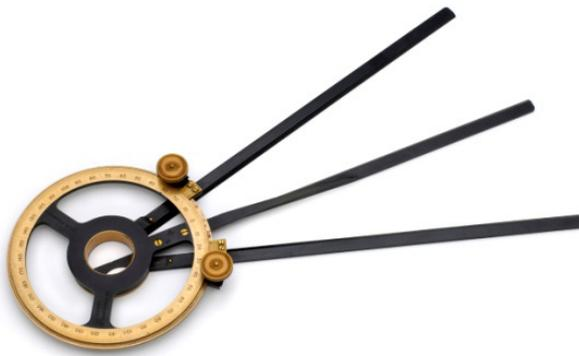
It is also possible to use a station pointer, as in this 1910 example, which is independent of the compass. One arm is pointed to each of the three points on land, and then it is moved on the chart so that it touches all three and the centre is over the ship's position.
