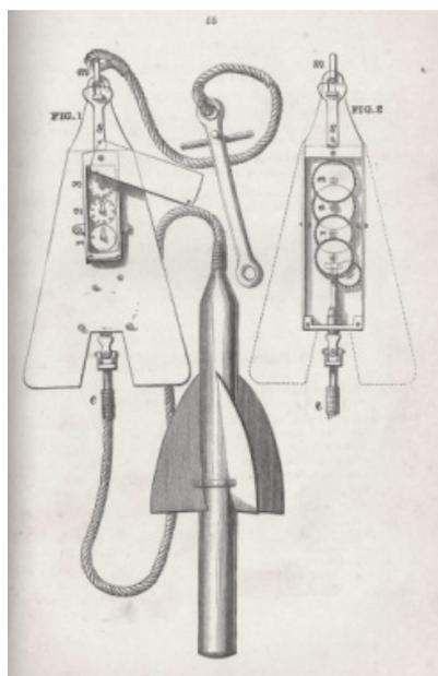
*A patent log, showing the line and impeller
