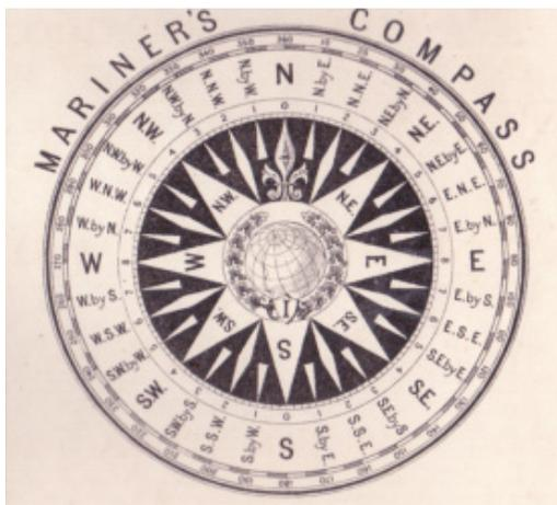
*Modern compasses are marked in degrees, with 360 or 0 degrees being north, and 180 degrees due south.*
