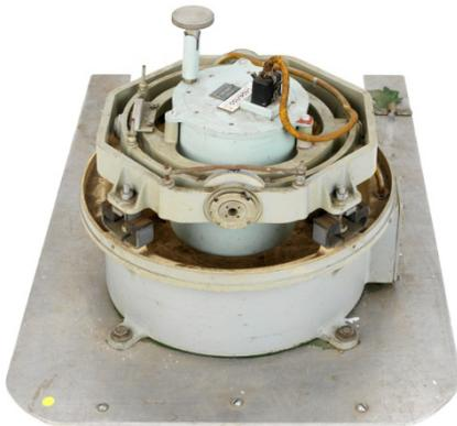
*The gyro compass has the advantage that it is not subject to deviation and variation, but it needs a good deal of maintenance and is mostly used on larger vessels. This example dates from c 1952 and is shown without the compass card on top to expose the mechanism.*
