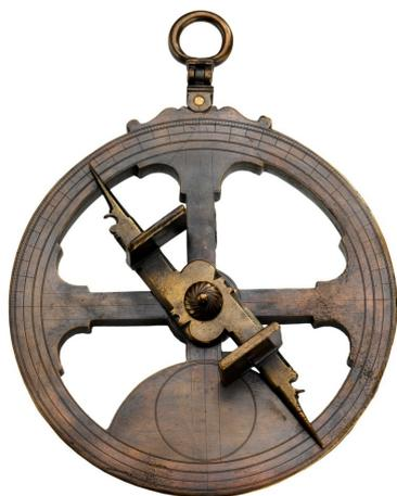
The astrolabe solved the problem of the sun by letting it shine through two holes in the moveable arm in the centre. It was heavy to keep it vertical when suspended, but it was difficult to use in a moving ship.
