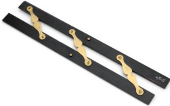
*A 19th-century parallel rule used to transfer lines on a chart.*
