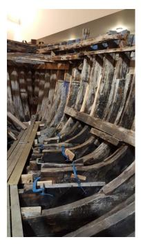
Along with this, rigging wires are being added to support the starboard side of the boat. The rigging wires will be placed throughout the boat to ensure the weight is proportioned throughout the boat. I was then shown how to add the rigging wires into the frames of the boat. I feel I am enjoying working in the boatyard more and more each week as I am constantly learning new skills.
