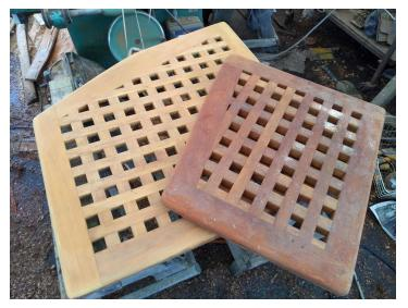
Who doesn't love a good before and after! These grating pieces out of the heads on Pellew are an example of some of the projects I've completed this month. They have been in the boat for some time and are in need of some TLC after being covered in dust and spots of paint. The one on the right is straight out of Pellew and the one on the left is after being sanded and ready for a fresh coat of oil. Quite the difference!
