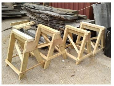
With so many boats being worked on, we knew work surfaces and areas were going to be in high demand so I was tasked with building some new trestles. Ned showed me the basics and gave me a power/shop tool refresher. I used an existing trestle as a template, taking measurements and using my bevel gauge to find the angles. I made one as a prototype and then cut enough parts to build 3 more. I enjoyed this challenge and they've already been put to good use!
