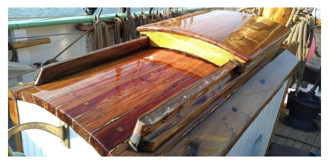
Other jobs included sanding and varnishing the top of the companionway, capping rails and coach roof, we achieved a really lovely finish by sanding with 120 grit, cleaning with spirits and then applying the varnish with a good quality brush. Small areas at a time were covered in a crosshatch pattern before brushing in the direction of the grain. We also oiled all of the deadeyes with linseed oil, being sure to get into all of the nooks and crannies and wiping any drips off the paintwork below.
