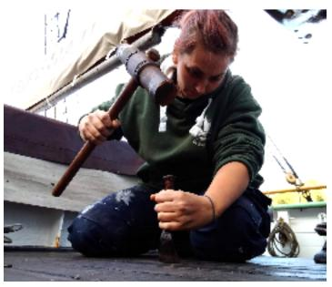
During my final week with the ship, Nikki showed me how to "harden up" the caulking seams in the deck ahead of the application of new pitch. I started by raking out the seam a little, then used caulking irons and a mallet to carefully compact what remained. Meanwhile the new resin was heated and once runny enough it was poured into the seams - the smell of hot pitch tar was incredible! The next day the excess was scraped off the deck, leaving neat, shiny black seams.
