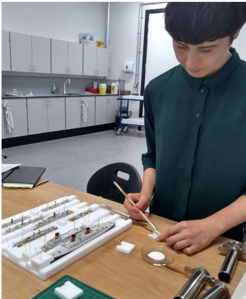
Left: Glueing plastazote foam to make stoppers for each end of the models.
