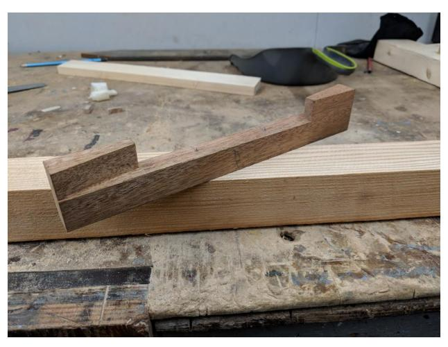
Back in the tropical paradise that is our workshop at the International Boatbuilding Training College (IBTC), we learned about spar making. First, we made a spar gauge with a ratio of 7:10:7 for marking out how much of the corners should be planed off. We use this ratio to assure that the faces all end up the same size. Next, a long piece of timber is planned true all round and marked out with the gauge, and then planed into a regular octagonal prism.
