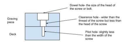
holes is so that the screw effectively 'clamps' the graving piece to the deck. Since the thread is gripping inside the pilot hole and the head can't fit through the clearance hole the screw pulls the wood down squeezing them together.
