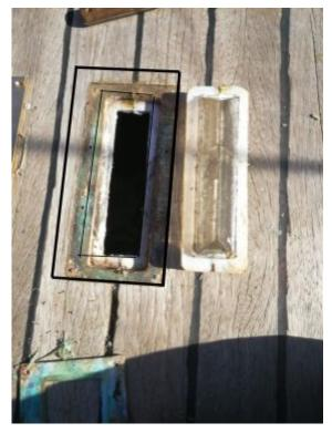
consuming was to create a 3mm recess into the deck for the brass cover plate to rest and not stick out of the deck too high. It was challenging because I needed to fair it so that it was uniformly flat the whole way around, I did this using chisels and skills I learned from ibtc joinery class. Once the on deck part was done I went down below and created bevels into
