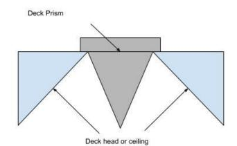
Once I was finished with all the wood shaping I cleaned up the area, used silicone to stick the prism into place then screwed in the brass cover plate.
