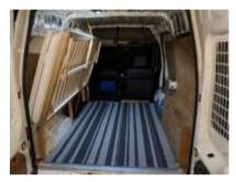
Completely stripped out and making some patterns out of cardboard to fit insulation RHS. I marked out some 'stations' on the floor and took some measurements off those to help with planning the layout.
