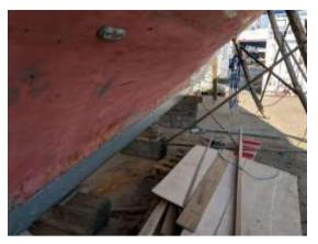
Jolie Brise has a cast iron keel, acting as external ballast. I gave this a going-over with an electric wire brush. There was some bad pitting where the water had got behind the paint. The whole thing was then cleaned off and treated with two coats of Primocon.
