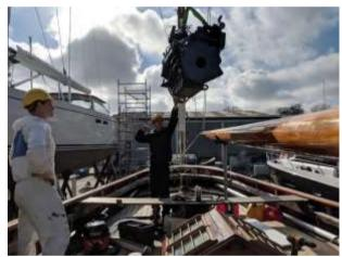
We had the engine craned back into place and bolted it down. One of the coach bolts wouldn't screw down as the wood below it was rotten, so we doweled the hole with some iroko and epoxy to drill a new screw hole later.
