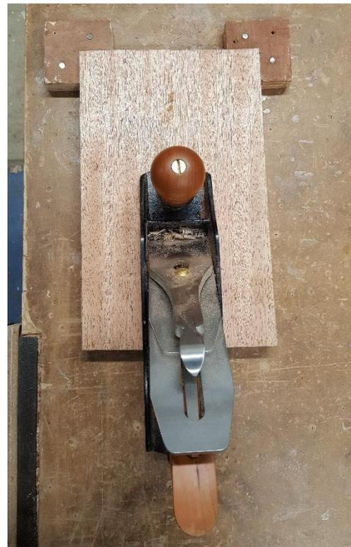
Making the bench hook, using the number 4 plane to ensure the surface is smooth and an even edge.
