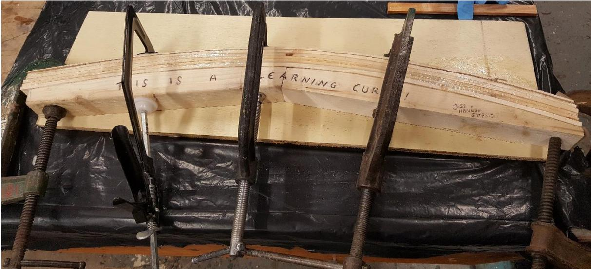
The planks of wood that I had laminated and glued together, clamped down to keep shape until the glue had dried.
