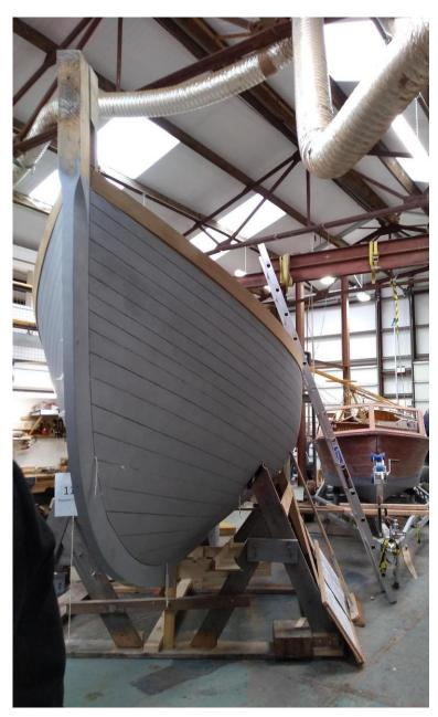
go at 'roving' — a method of riveting clinker boat planks together.
