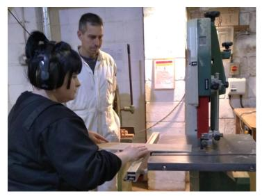
We started by working out the angle of the curve and made a plywood template which was transferred onto a solid timber big enough to hold the work and accept several clamps. This was shaped on the bandsaw and mounted onto a board to form a mold. We started with the lamination: layering thin strips of wood and glue and clamping it
