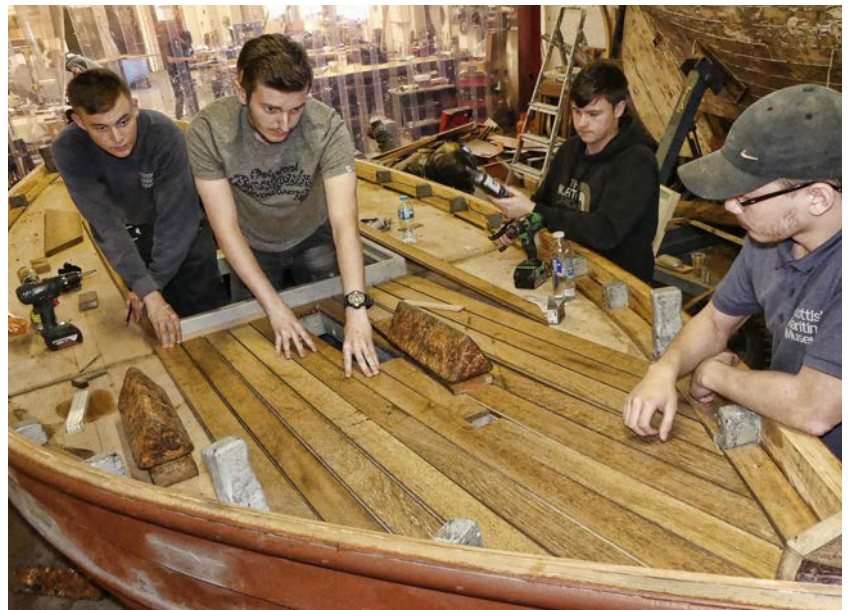
Planking the deck, by Alan Kempster.
