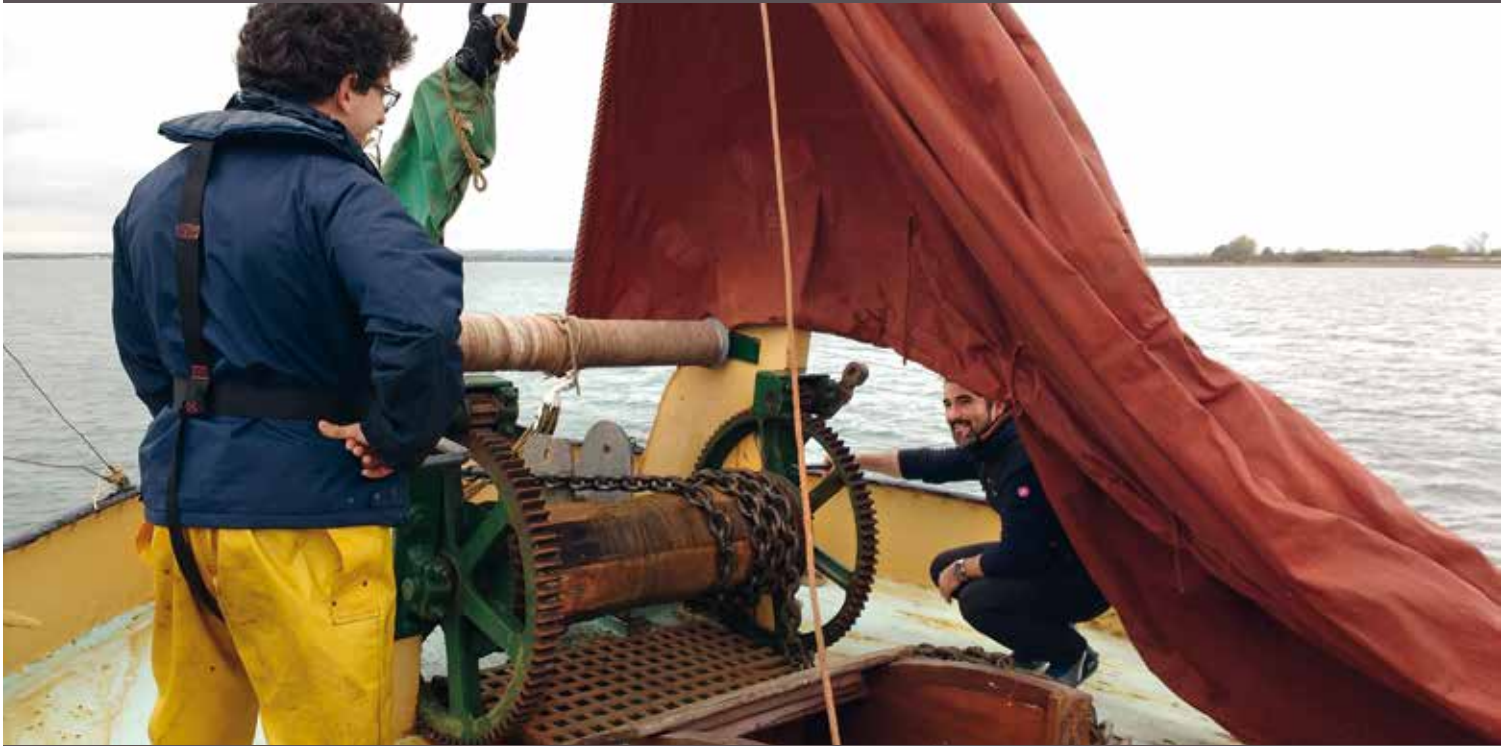
When anchoring, the windlass and chain need to be fully prepared to ensure free-flow. Photograph by Gabriel Clarke.
