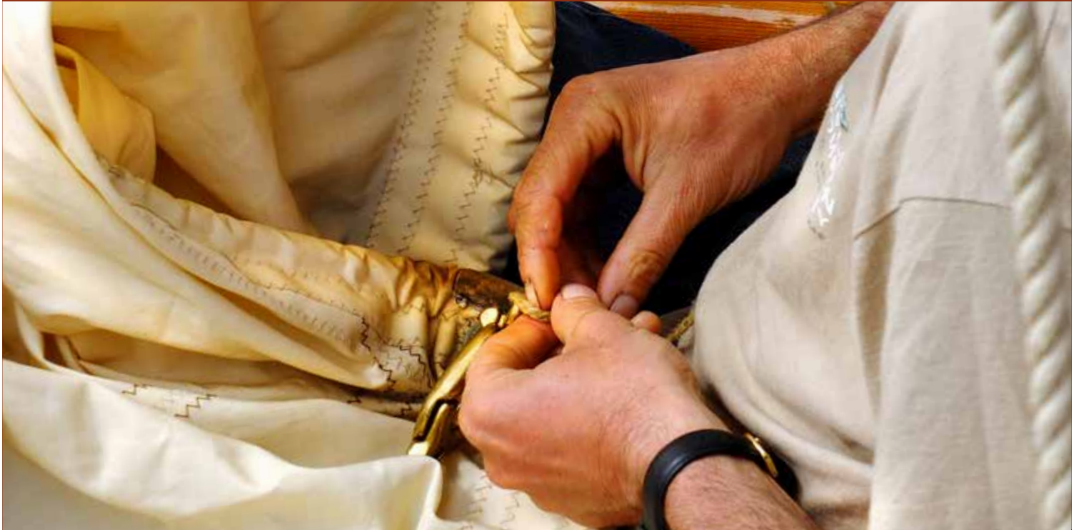
Replacing the hanks helps the sail to last. Photograph by Henry Faire.
