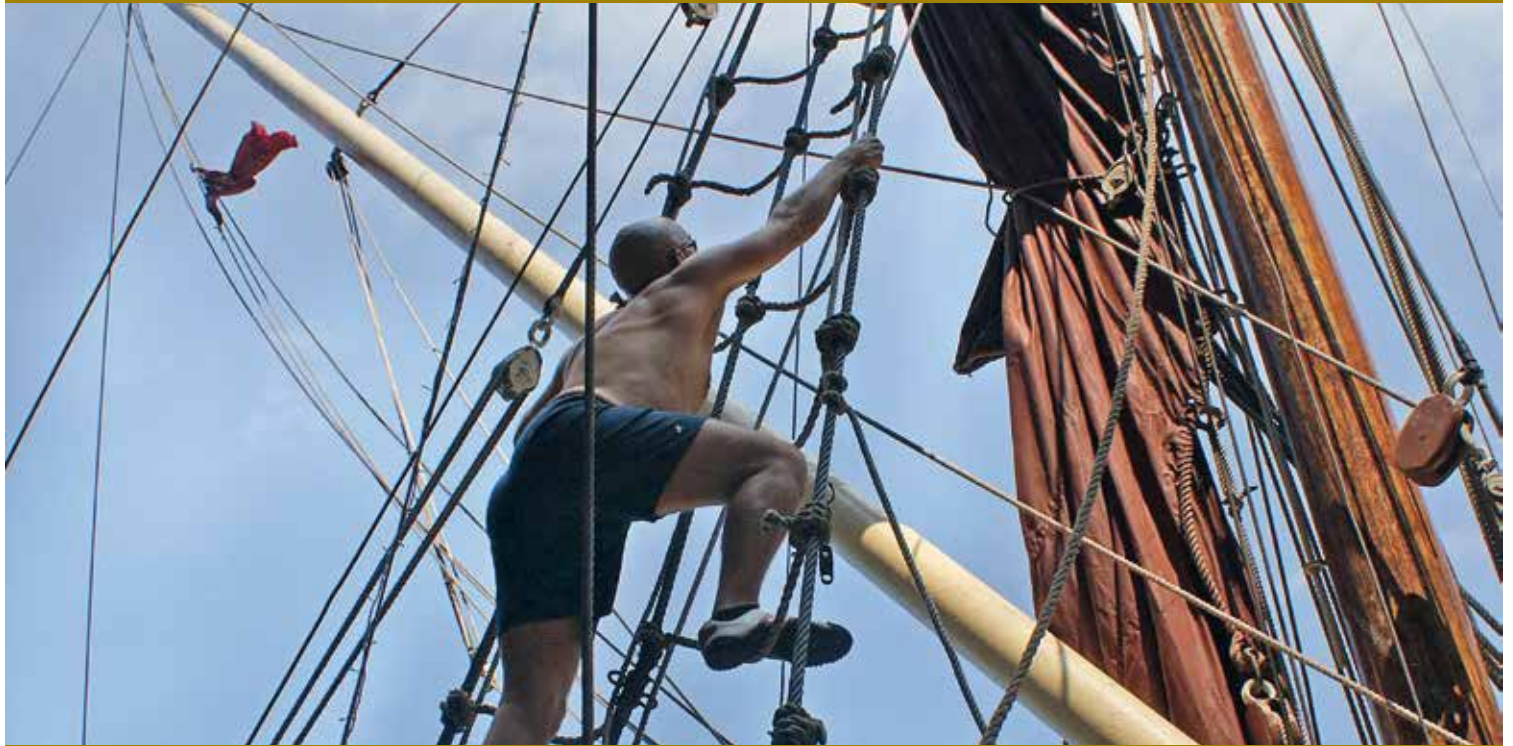
Ratlines provide a quick way aloft to deal with any issues when hoisting, reducing or stowing sails. Photograph by Alistair Sommerlad.
