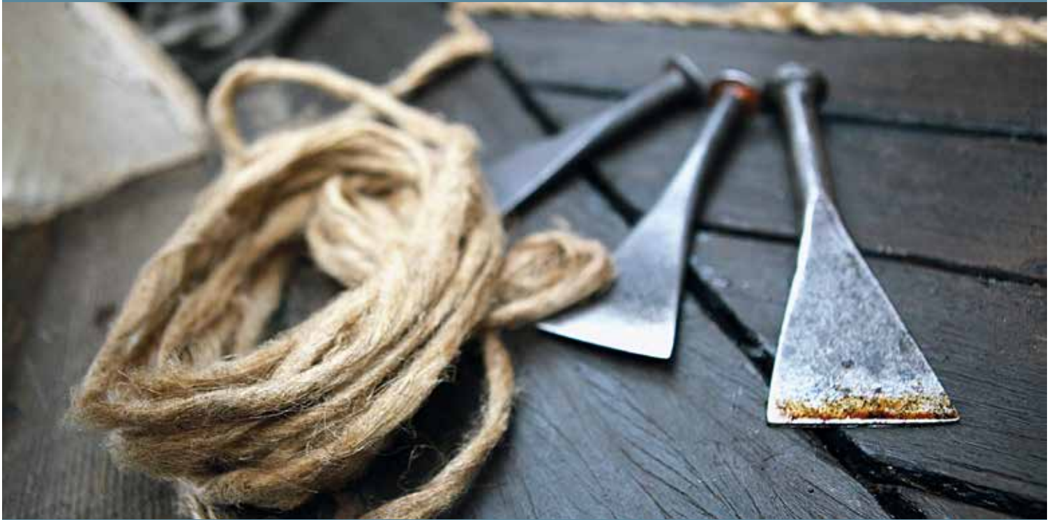
It's important to have the right tools when caulking the deck. Photograph by Bryony Stokes.
