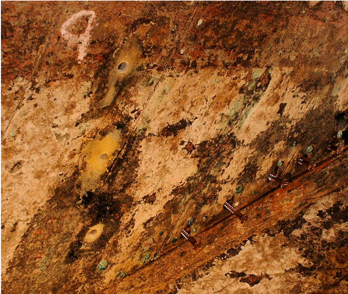
Fig.7b The re-drilled floor fastening holes having first been filled with epoxy resin/filler. The silicon bronze screws are there to replace the hood end naval brass screws that were pitted.
