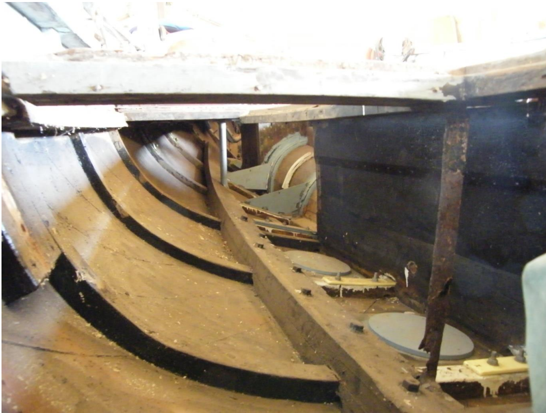
Fig.6 View from further forward, starboard side. The dark area to the right is the outer surface of the engine compartment. The circular disks blank off the hull skin end of the relieving tubes. These will eventually be through-bolted to the hull. Between the disks the new steel outboard ends of the engine compartment floors can be seen through-bolted to the frames and hull skins. The large section timber running fore and aft is the bilge stringer.
