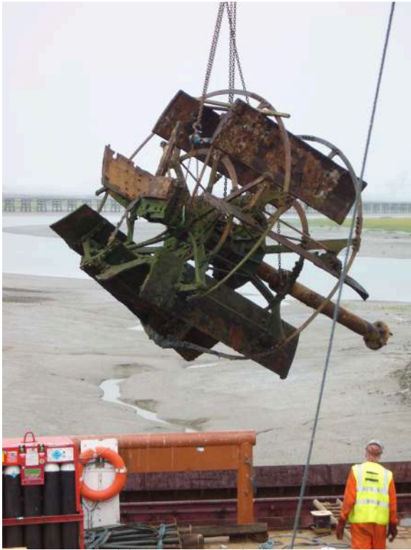
Hoisting paddle wheel and shaft clear of hull. Later rebuilt and reinstalled (W. Davies)
